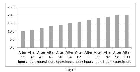
**Fig.** (9-10) shows the degree of absorbing of the stone cube with the material of SILRES BS OH 100.
