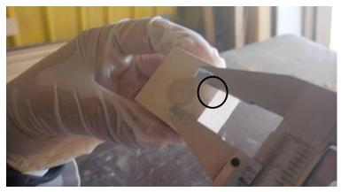
Fig. 11 Measurement of the diameter of the dispersed consolidation materials.
