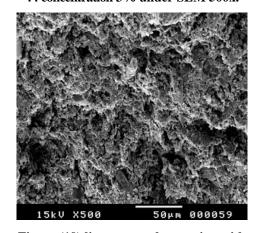
Figure (19) limestone cube treating with (paraloid B72 concentration 3%), and Ca (OH)<sub>2</sub> /polymer nanocomposites under SEM 500x.
