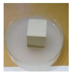
Fig. 2 Showing Immersion consolidation process
