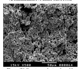
Figure (20) limestone cube treating with (paraloid B44 concentration 3%), and Ca (OH)<sub>2</sub> /polymer nanocomposites under SEM 500x.
