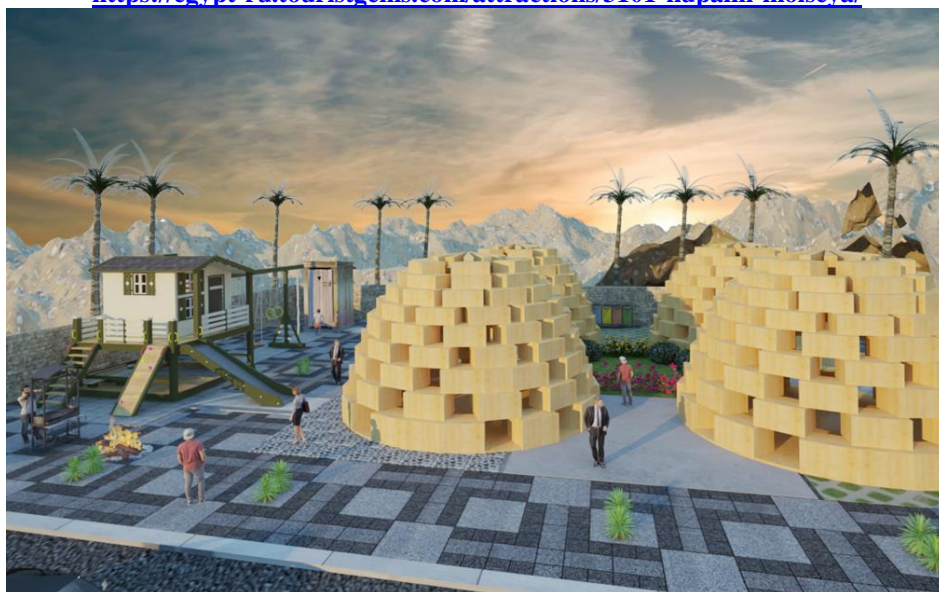
Figure (19) External perspective designed by the researcher – in which there is the idea of dividing the cafeteria area to four domes inside which there are tables and chairs and counters, also playing area for children, baths; there is also a landscape division and outer floors planning.
