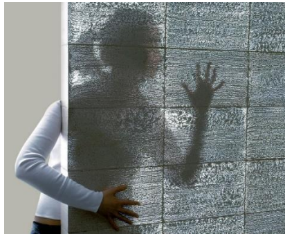
Figure 17 Translucent Concrete partition
