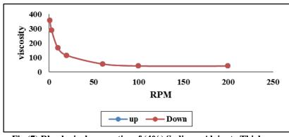
Fig (7) Rheological properties of (4%) Sodiume Alginate Thickener
