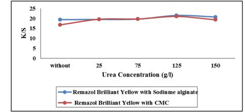
Fig (2) Effect of Urea concentration of Sodiume alginate and CMC printing paste on K/S of Remazol Brilliant yellow
