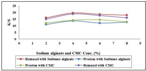
Fig (1) Effect of Sodiume alginate and CMC concentration on K/S for both reactive dyes
