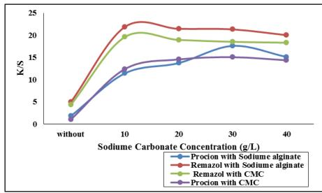
Fig (4) Effect of Sodiume carbonate concentration of Sodiume alginate and CMC printing paste on K/S for both reactive dyes
