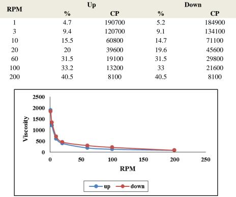
Fig (8) Rheological properties of (4%) CMC Thickener
