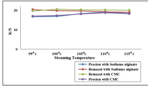
Fig (5) Effect of Steaming temperature of Sodiume alginate and CMC printing paste on K/S for both reactive dyes
