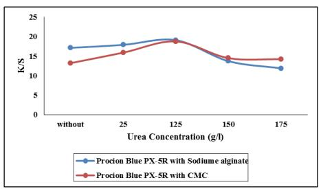
Fig (3) Effect of Urea concentration of Sodiume alginate and CMC printing paste on K/S of Procion Blue PX-5R
