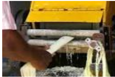
Fig.2 Extraction of fibers by rolling process
