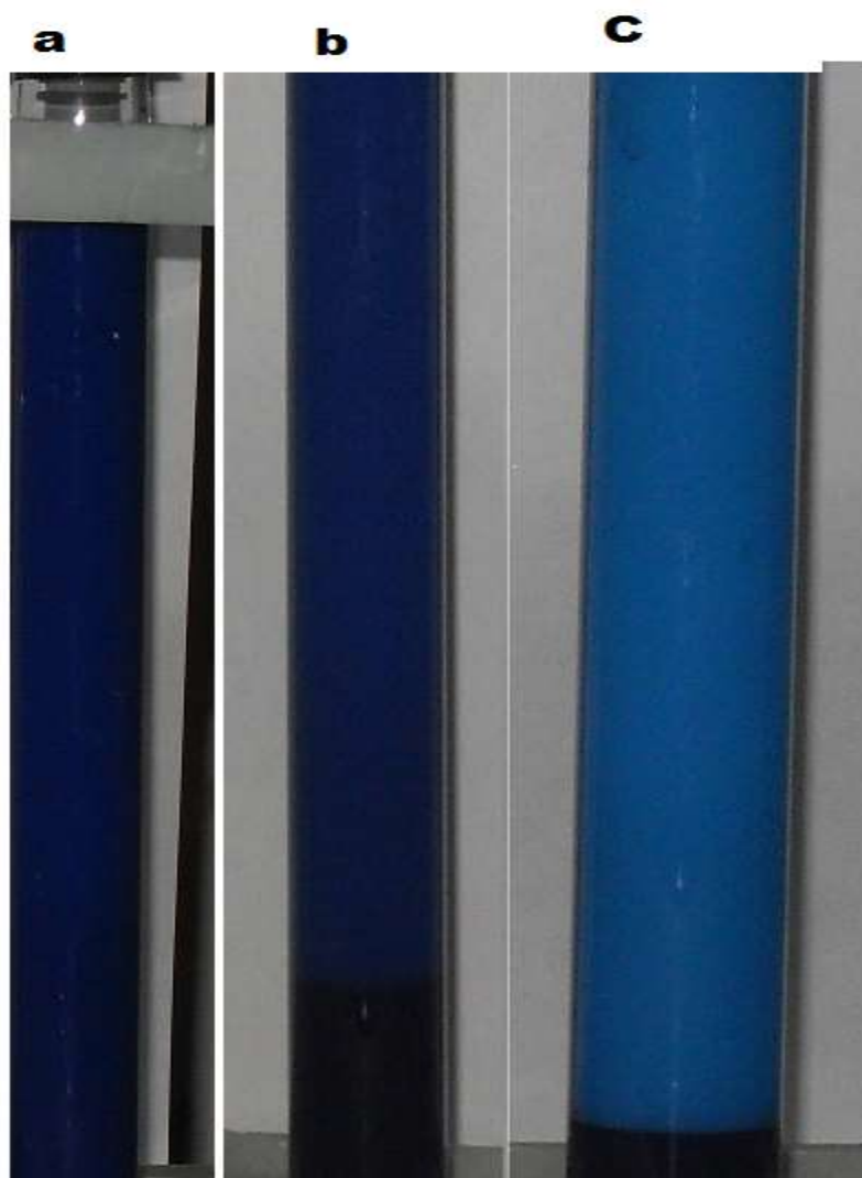
Fig.1. Photograph of shelf life stability of (a) APSV encapsulated pigment; (b) APSM encapsulated pigment and (c) Nanoscle C.I. Pigment blue 15:3, after 15 days of storage at RT.
