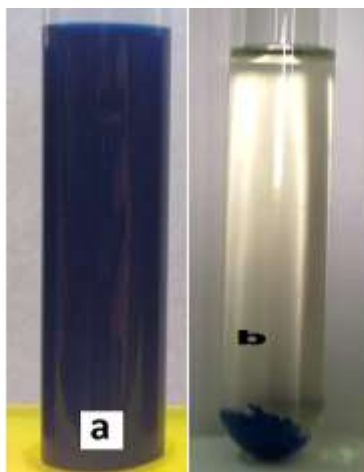
Fig. 5. Digital photograph of: (a) original PB15:3 and (b) encapsulated PB15:3 ultra-centrifuged with acetone for 30 min.
