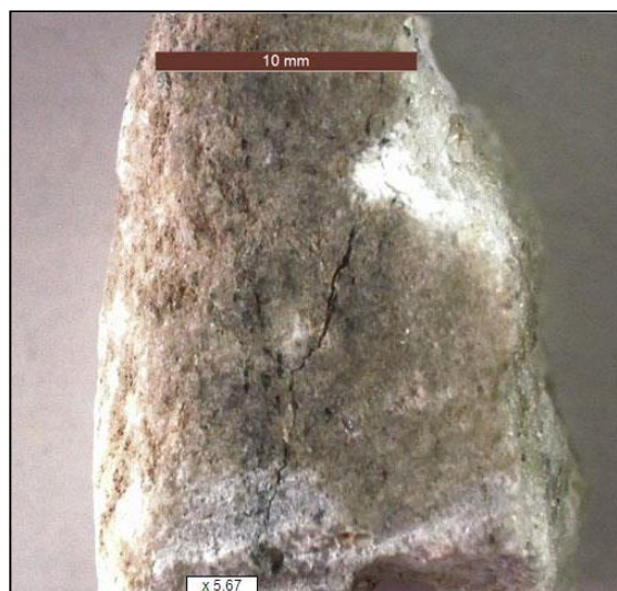
Figure 9. Cracks and gaps on the marble surface (stereomicroscope)
