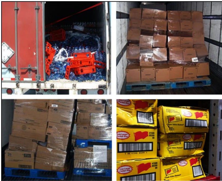
Figure 1: boxes damage during shipping due to stacking over-load Source: (13)
