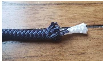
Figure (10) Double braided rope construction.
