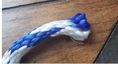
Figure (9) single braided rope construction.
