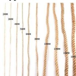
Figure (11) Jute rope cord.
