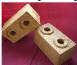
Fig (38) Lego Blocks from Straw [41].
