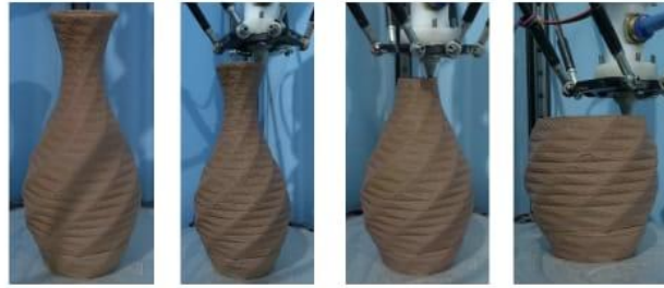
Figure 11 illustrates the process of shaping Aswan clay, firing it, and transforming it into three-dimensional ceramics. clay ( Rasha fawzy –Ibrahim Eldesoky- An Applied for the design and implementation of ceramic 3D printer- the International Journal of Educational Sciences at South Valley University-p244 )
