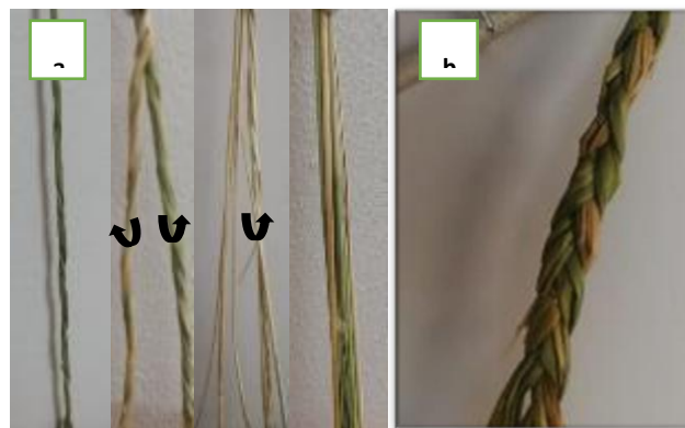
FIG. 11: ROPES MANUFACTURING A) TWINNING PROCESS B)
