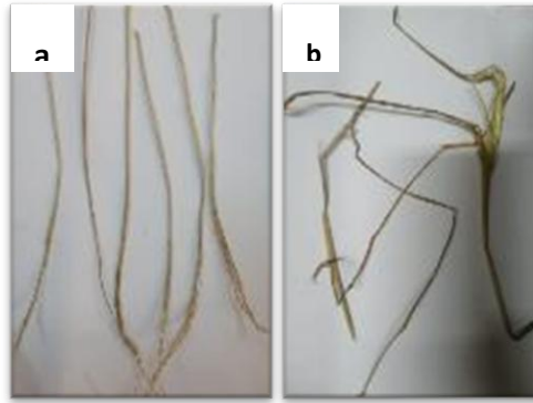
FIG. 10: SELECTING A GOOD RICE STRAW FIBERS: A) HIGH QUALITY FIBERS B) LOW QUALITY FIBERS
