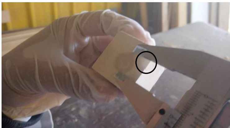
Fig. 11 Measurement of the diameter of the dispersed consolidation materials.
