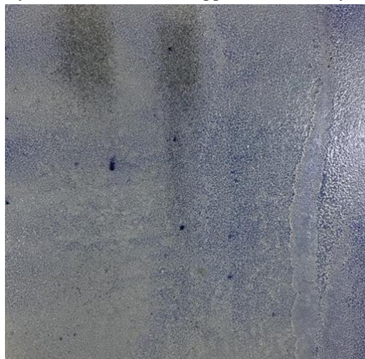
The firing at 1170 and the fire cycle 38 minutes and application with salt-colored emulsion by spraying Experiment (16).
