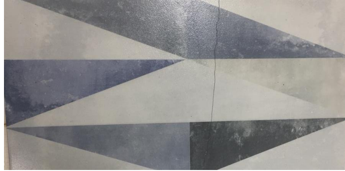
B. Application by spraying the salt emulsion under the printed design by the ink jet method.
