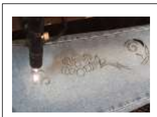
The laser beam cuts the cloth according to the design
