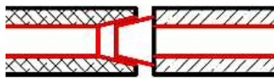
Figure (2) Installation of parts of self-installed glass accessories (vertical diagram of dovetailing the two units)
