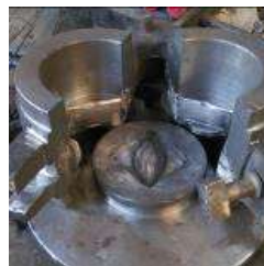
Figure (6) Shape of the mold manufacturing of blowing mold to match the compression method for the various bases that are used
