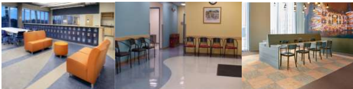
Figure (1) shows the use of natural floor linoleum in public places, indicating the strength of the resistance and corrosion with different colors and effects, and the possibility of the work of different designs is a material of high durability and fire resistance and flame retardant, antibacterial, and available more than 100 colors.
