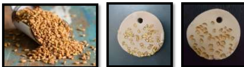
Fire temperature 950 ° C- Appearance of seed form The color is reddish brown due to the iron element in the seed structure.
