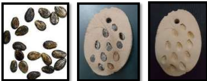
Fire temperature 950 ° C- Appearance of seed form The color is reddish brown and light green black due to the iron and copper elements in the seed structure.
