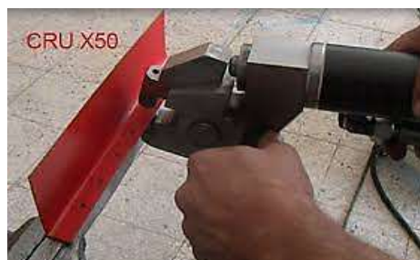
Figure (7) A handheld tool for clinching joining of metal furniture parts (9)
